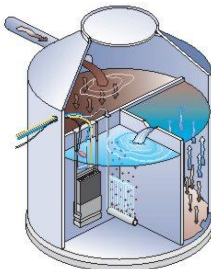
Figure 35. MembraneClearBox of the German company Huber, the first certified small size membrane bioreactor in Germany ( www.huber.de )
